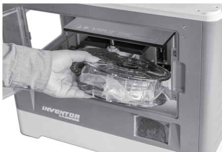
13. Take out filament first and then remove foam.
