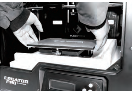
12. Elevate the build plate to its limit with care.
