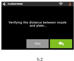
(5-2) After tapping **[Yes]**, the extruder starts to move towards the first point and the plate moves up and down to verify the distance between nozzle and plate.
