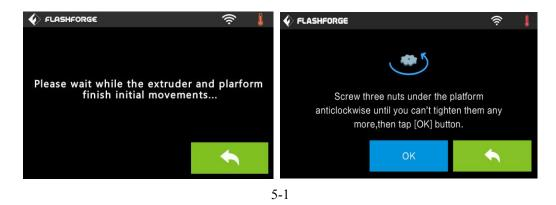
(5-1) Tap [Tools] - [Level] on your GuiderII touch screen. Please wait while the extruder and platform finish initial movements. After that, operate according to the guide on the touch screen.
