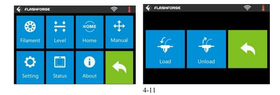
(4-11) Tap [Tool]-[Unload] and the extruder starts heating up.
