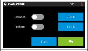
Tap the **[Preheat]** button to enter the preheat interface. Tap the **[Start]** button to heat up to the setting temperature.
